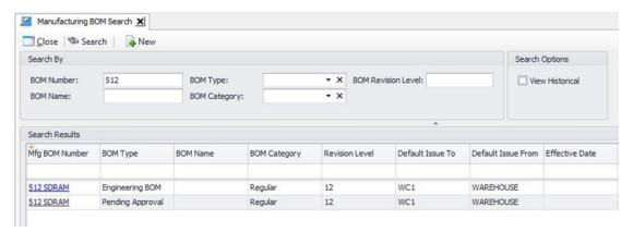
The user opens the 512 SDRAM Pending Approval BOM. An **Approve** button is on the taskbar if the user has the Security: **Can Approve BOMs** enabled.
