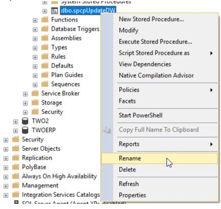
$Add \ the \ text \ ".bak" \ to \ the \ end \ of \ the \ procedure \ name, \ indicating \ that \ the \ custom \ procedure \ is \ now \ a \ backup.$
