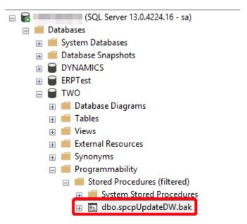
Renaming the procedure effectively changes its identity, causing the default procedure to no longer "see" the existence of a matching custom procedure. To begin using the custom procedure again, simply rename it, removing the ".bak."
